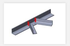
Always design stiffeners and gusset plates so that zinc cannot be trapped in corners.
