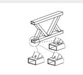
Place the holes as close to corners as possible! As well proper direction of holes should be considered. It heps the galvanizer if the holes all drain in the same direction. This avoids manipulating and turning of the article with risk of damage or trapping zinc in pockets.
