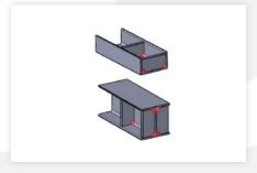
On universal sections or channels, make sure that the corners of stiffeners are cut to allow zinc to drain through.
