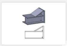
When designing right-angled supports or similar structures, holes should be drilled in places indicated in the drawing.
