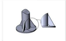
When you use external props, for instance, between a base plate and a vertical element, make sure the prop is cropped to allow zinc to drain freely.
