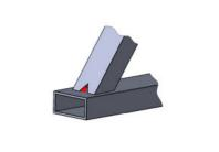
"V"-type notch is a good alternative to drilled holes.
