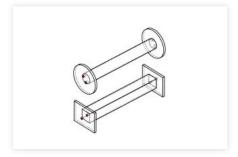
When designing or producing structural hollow structures, remember to provide for each separate element appropriate drainage. The technological holes must be located at the ends of the pipes on opposite sides diagonally.
