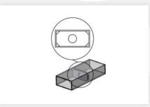
When using internal diaphragm, make sure the corners of it are cut. On larger RHS use a stiffener with a central hole as well as cut corners. NEVER arrange a plate that blocks the entire cross section. It may be dangerous during hot dip galvanizing. (One may happen to be unpleasantly surprised when receiving an invoice if the entire section has filled with zinc which cannot escape!)
